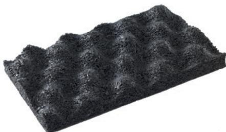
The RailMat **Ballast Mat Damper** is a vibration damper made of recycled rubber that is installed under the ballast of a railroad. It reduces vibrations of ballasted tracks in urban areas (up to -20 dB @ 63 Hz).
